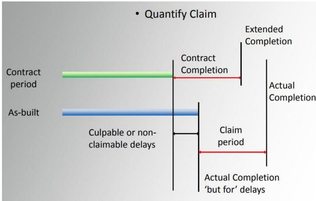
Figure 52 Collapsed As-Built (Or But-For) Analysis Method
